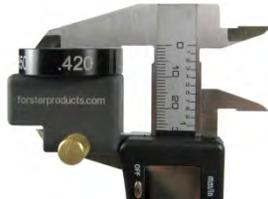
**Step 5.** Open the caliper. Insert the case shoulder into the selected datum diameter.
