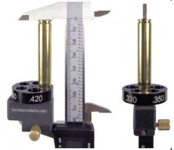
**Step 7:** Measure the other four cases, record the measurements and calculate the average. *Remember: repeatability is important when taking measurements.*
