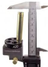
**Step 6.** Rotate the case to remove slack while centering the case along the measurement axis. Ensure the case is perpendicular to the Dial. Gently, but firmly, tighten the caliper on the case head and record the measurement in Table 3.
