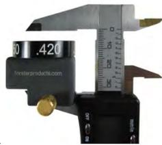
**Step 4.** Gently, but firmly, close the caliper on the Datum Dial. Tighten the Thumbscrew. Zero out the caliper.
