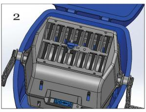
Put your mixed caliber brass into the basket and close the latch. Use the cartridge case that you want to sort out first as a guide to set the shutter. Start with the shutter in the closed position (image 3) and open the shutter until the brass falls into the basket. Place the next size (caliber) brass for sorting onto the shutter to make sure it does not fall into the basket. Repeat the calibration process with each successive size
