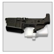
Support the trigger guard "ears" while installing or removing a trigger guard.
