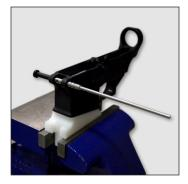
Use the other end of the pin driver to install the takedown pins / springs
