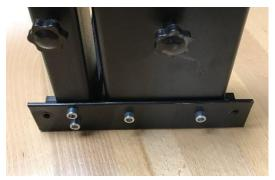
2. Attach the steel base to the outside of the upright frame using the thumb screws:
