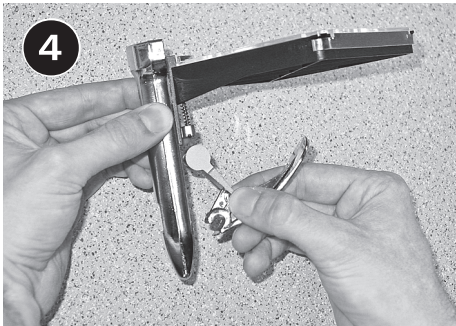
4 Lubricate metal parts at wear points with grease or Vaseline. Reinstall into body.
