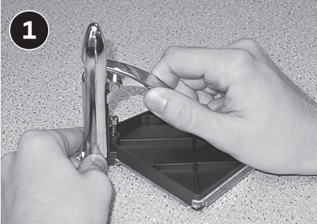
1 Remove lever and connecting rod by pulling lever towards the tray.
