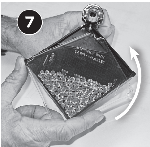
7 Tip tool so primers slide away from body. Be sure no primers remain on the NO PRIMER ZONE. Hook tray cover as shown, slide towards handle, and make sure small tab on cover engages the trough.
