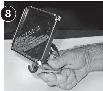
8 Hold tool at 45° from horizontal; rotate tool clockwise to fill feed rail.
