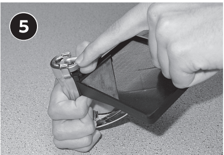
5 Push down on tray—install appropriate shell holder. Slide tray upward until it contacts bottom of shell holder.
