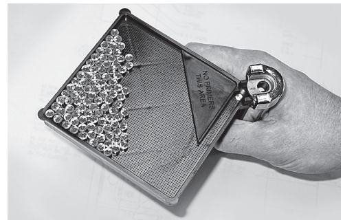
6 Place a box of 100 primers in the tray. Remove box and shake the tray side to side to upright all the primers.
