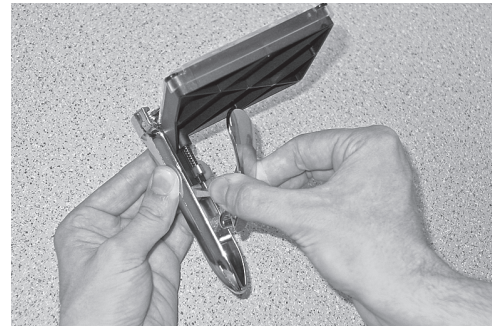
4 Lubricate metal parts at wear points with grease or Vaseline. Reinstall into body.
