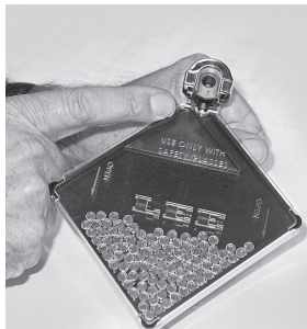
7 Tip tool so primers slide away from body. Be sure no primers remain on the NO PRIMER ZONE. Hook tray cover as shown, slide towards handle, and make sure small tab on cover engages the trough.
