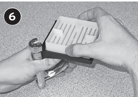
6 Place a box of 100 primers in the tray. Remove box and shake the tray side to side to upright all the primers.
