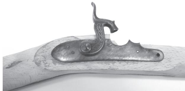
2. Once the lock assembly is in place visually verify that the screw holes line up. If holes are not perfectly aligned, enlarge one or both stock holes with a round file or drill to permit alignment. Screws should be snug against the barrel.
