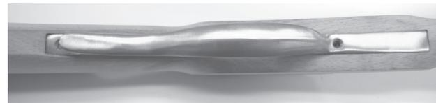
3. Place the Trigger assembly into its cut out slot. Here again you want a snug fit but not so tight that it has to be forced in.
