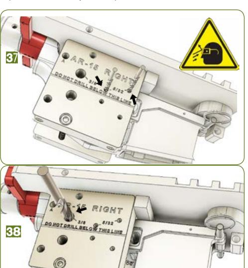
TIP: If you milled a raw lower, do not apply a finish coat to the lower until after a lower parts kit is installed and a function test performed. If you milled an anodized or Cerakoted lower, it is not necessary to apply a finish coat to the raw milled aluminum area.
