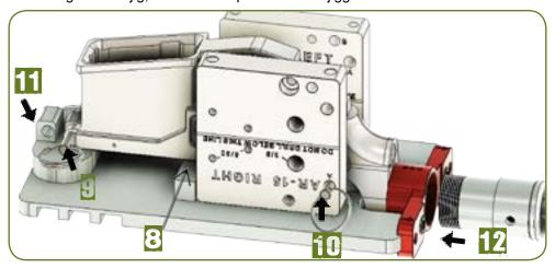
Tilt the jig assembly onto it's front end (Fig. 13). Tighten the side plate bolts while pressing and holding the side plates flush against the center alignment bar to ensure perfect square alignment of the side plates.
