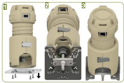
Reuse the router's screws to loosely attach the router attachment plate. If the router came with tapered screws, replace them with screws that have a flat inner face. The metric M4-0.7 pan head screws provided with your jig will fit most compact routers. Make sure the thread pitch matches that of the router before attempting to use the screws. Do not tighten the screws at this time. **Do not use screws which have a conical tapering inner face with the router attachment plate.**
