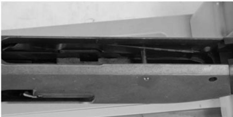
The loose shell latch positioned in the receiver for restaking.
