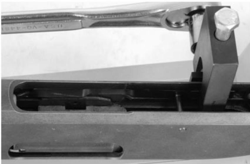
**The staking tool in the proper position.**
