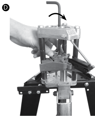
Loosen turning clockwise with a 1/4 inch hex key while holding the shell plate
