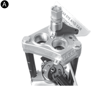
Remove Smart Lock bushing from station 2.
