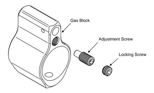
The Wilson Combat adjustable gas blocks are designed so that the shooter is able to restrict the gas flow and slow the cycling of the rifle. This achieves a lighter recoil impulse or corrects an overdriven rifle (such as with a fulltime suppressor). A full wide open gas block will have the locking screw flush with the front of the gas block after stopping it against the adjustment screw.
