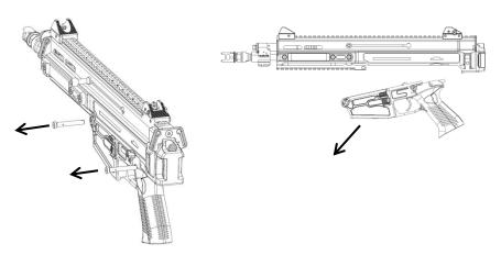
C. Press the disassembly button fully and remove the rear head by sliding downwards.
