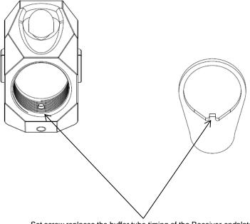
Set screw replaces the buffer tube timing of the Receiver endplate
