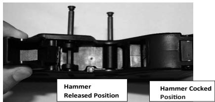
**\*\*\*Please note – Be sure the hammer is in the COCKED position before attempting to remove the Sear Housing Mechanism\*\*\***
