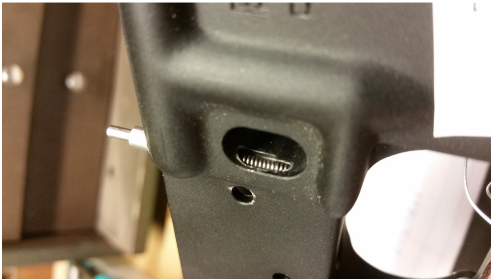
(Picture-2) Note: Both drills break through walls into pocket.
