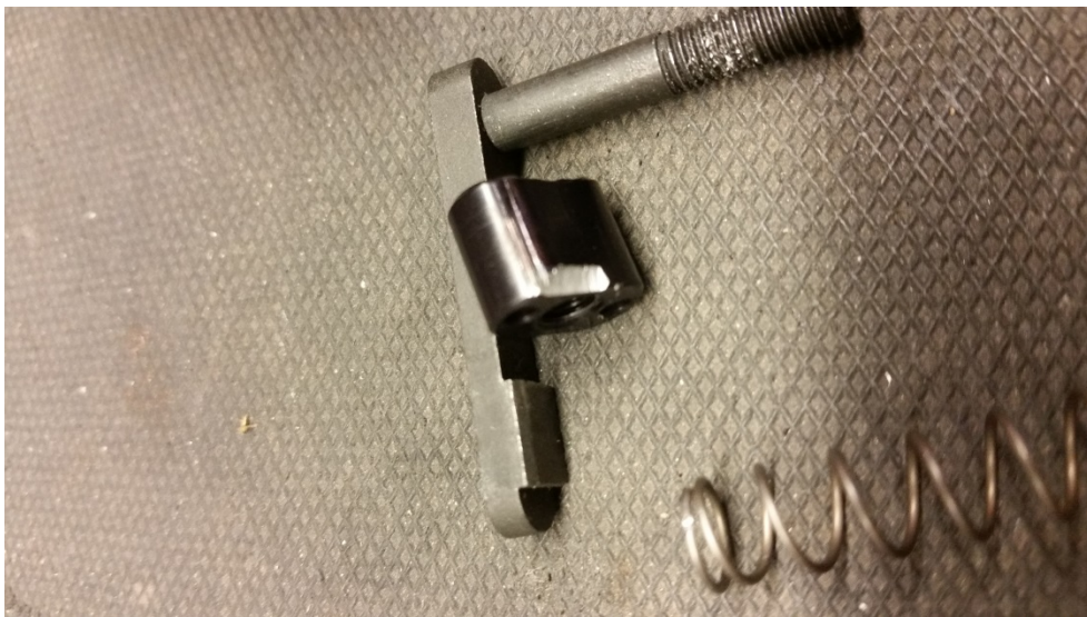
(Picture-3) Note: Drill notch on mag button. This cut creates locking / wear surface for pin.
