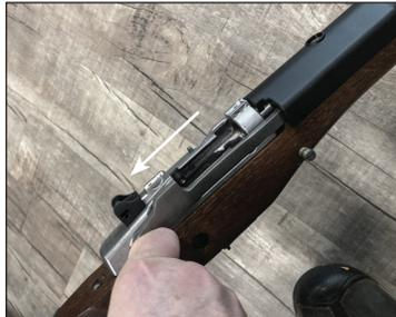
4. Invert the rifle so that the magazine well is facing up. Insert a 1/4" steel rod, punch, screwdriver, or other suitable instrument into the hole in the rear of the trigger guard. Lift up, using the tool as a lever to spring open the trigger guard from its latched position.
