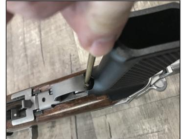
5. Remove the trigger housing assembly by carefully pulling it upward. Be careful not to damage the stock when removing or replacing the trigger housing.
