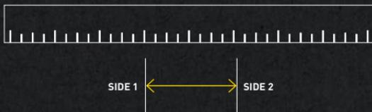
Use a ruler to measure the distance between the lines of each lens to determine the size of scope cover you need.
