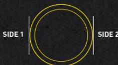
Stand your scope up on a piece of paper. Mark a line on each side of both the eyepiece & objective lenses.
