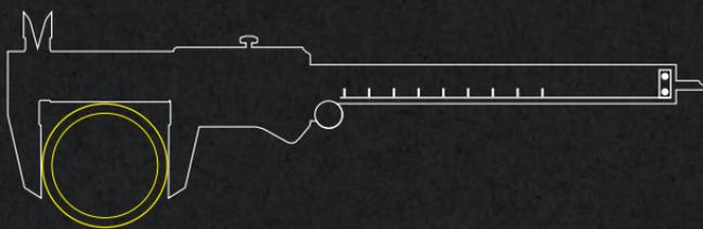
Use the calipers to measure the outside edge of the scope housing on both the eye piece and objective. You can measure in inches or millimeters.
