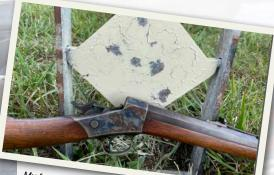
block to open, and then holds the breech block closed, as it rolls forward to fire. It's a simple action and very easy to operate with one hand.
