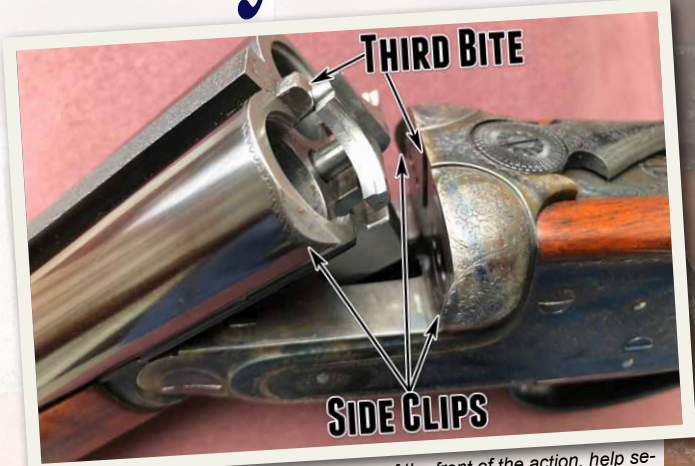
The side clips, protruding from both sides of the front of the action, help secure the barrels during firing; all three of the guns have these. In addition, the 20 gauge (above) features a "third bite".
