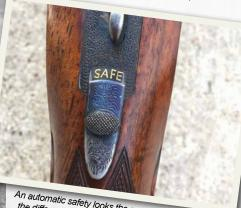
An automatic safety looks the same as any other safety, the difference is that it automatically moves back to the "safe" position every time the gun is opened. A great safety feature for a field gun, but a nuisance for many people, on the skeet, trap or clays range.
