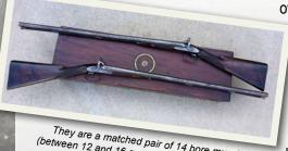
They are a matched pair of 14 bore muzzleloaders (between 12 and 16 gauge), with 30.5" length barrels.
