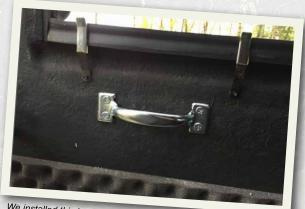
We installed this heavy-duty 6-1/2" door pull, secured with four ¼" rivets, for additional safety. It provides a secure grip on the inside of the door as we step up onto the landing and into the blind.
