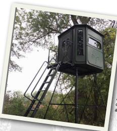
Looks pretty simple; just climb the ladder, open the door and walk into the blind. Now, add darkness and some snow, ice or frost on the steps—then safety can become more of an issue. We installed a second handrail on the left side, for additional safety.
