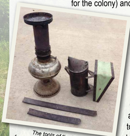
The tools of the trade -- simple but functional. The pry bars were broken leaf springs from an old car or buggy. Smoke from the smoker calmed the bees down.
