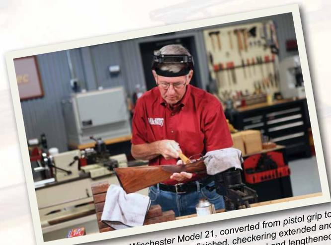
*Final assembly of a Winchester Model 21, converted from pistol grip to straight grip stock, with the stock refinished, checkering extended and trigger guard straightened and lengthened.*
