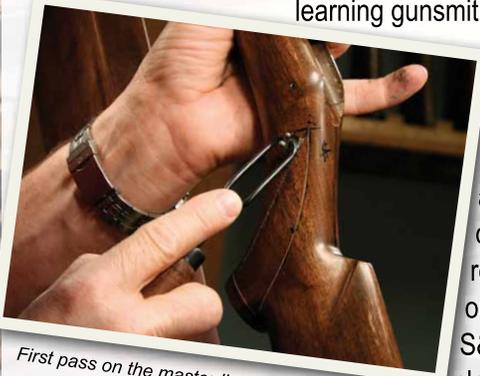
*First pass on the master lines is an early step in the checkering process.*
